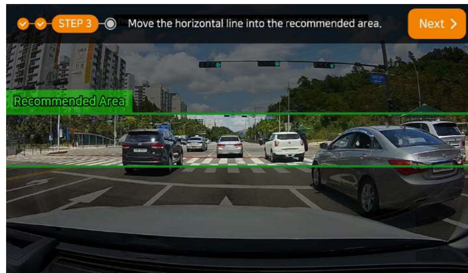
3. Adjust the angle of the front camera to align the horizon into the green area provided on the app screen.
